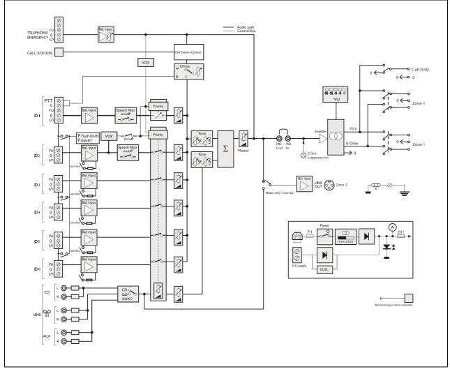
figure 2.1: Schematic overview of the Plena Mixer Amplifier
